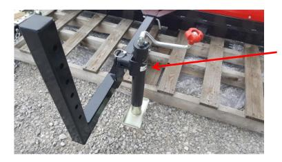
Step 13 Install the Jack onto the Steel Tongue.
